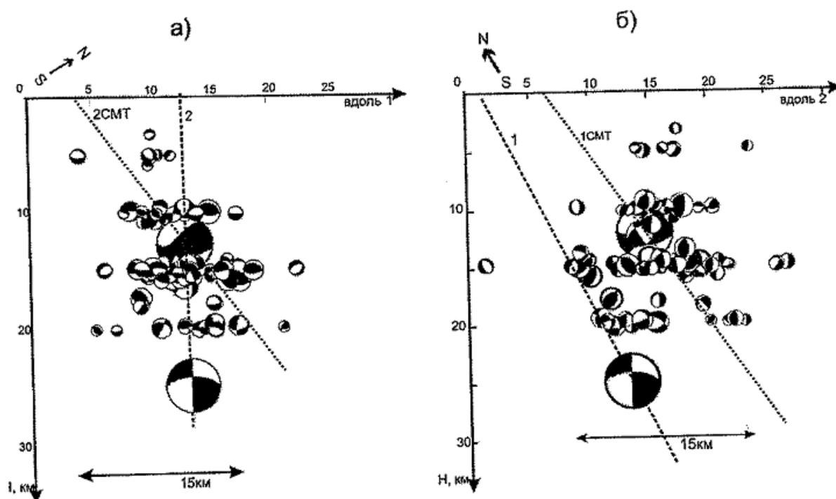
**Figure 8.** Depth section of the aftershock cloud of the earthquake occurred in 2009; a) – on the first nodal plane, b) – on the second nodal plane
