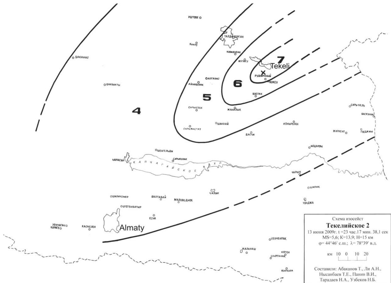
**Figure 11.** The isoseismal map of Tekeli earthquake of 13.06.2009
