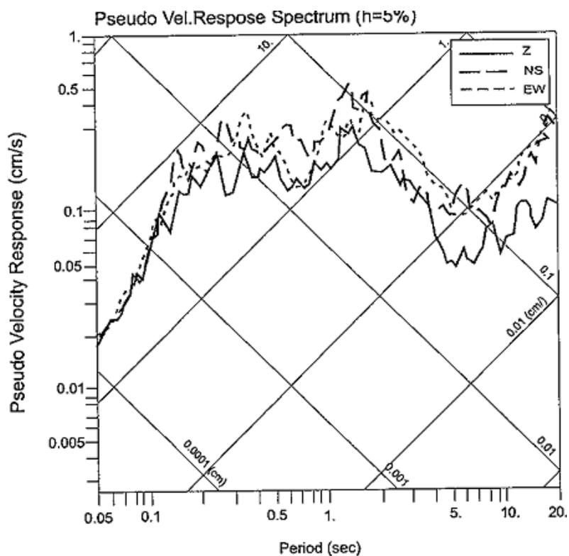
**Figure 14.** Response spectra by three components of the records from KNDC station**Table 3.** Parameters of strong motions of Tekeli earthquakes on the territory of Almaty
