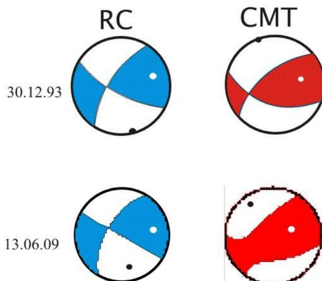
**Figure 4.** Stereograms of focal mechanisms of earthquakes occurred in 1993 and 2009 by data from regional MO catalogue and CMT catalogue.
